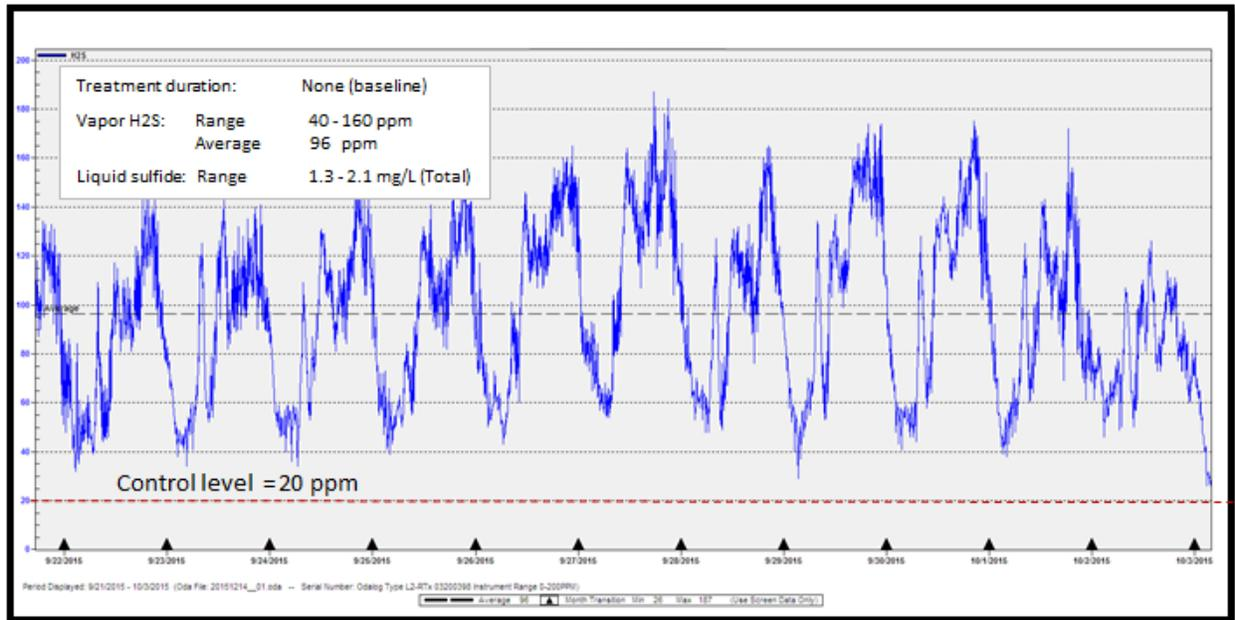
Figure 10 shows the results obtained by dosing nitrate at a rate of 29 gpd, or a ratio of approx. two gallons per lb-Sulfide. The effect was a substantial 80-90% reduction in H<sub>2</sub>S at the FM discharge, though there remained several hours of the day where control levels were exceeded by a factor of two or more. Increasing the nitrate feed rate to 39 gpd was able to consistently control H<sub>2</sub>S to the target level (Figure 11).
