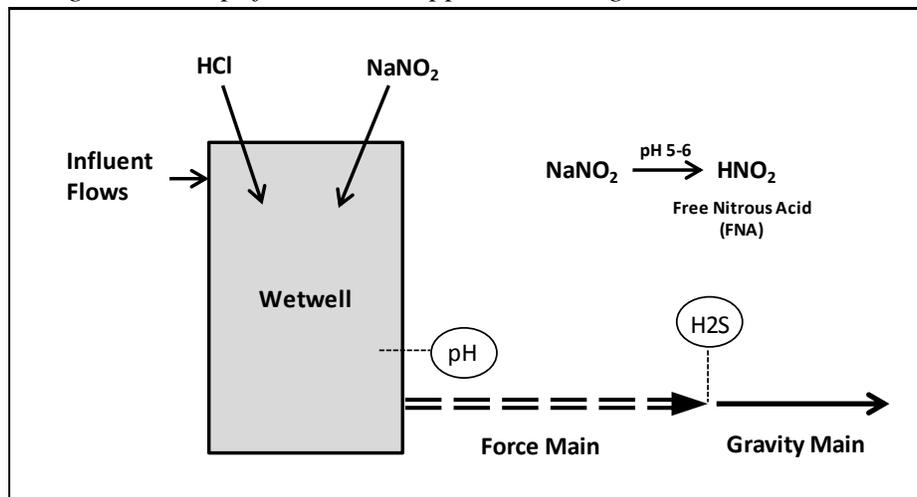
The equipment needed to apply the Cloevis technology consists of two subsystems supported by data acquisition and telemetry for remote operation. The first subsystem is the chemical storage and dosing module which, depending on sizing and site constraints, can be either stationary, temporary (for applying treatments), or completely mobile (contained). Figure 4 shows the temporary module used in the first case study.
