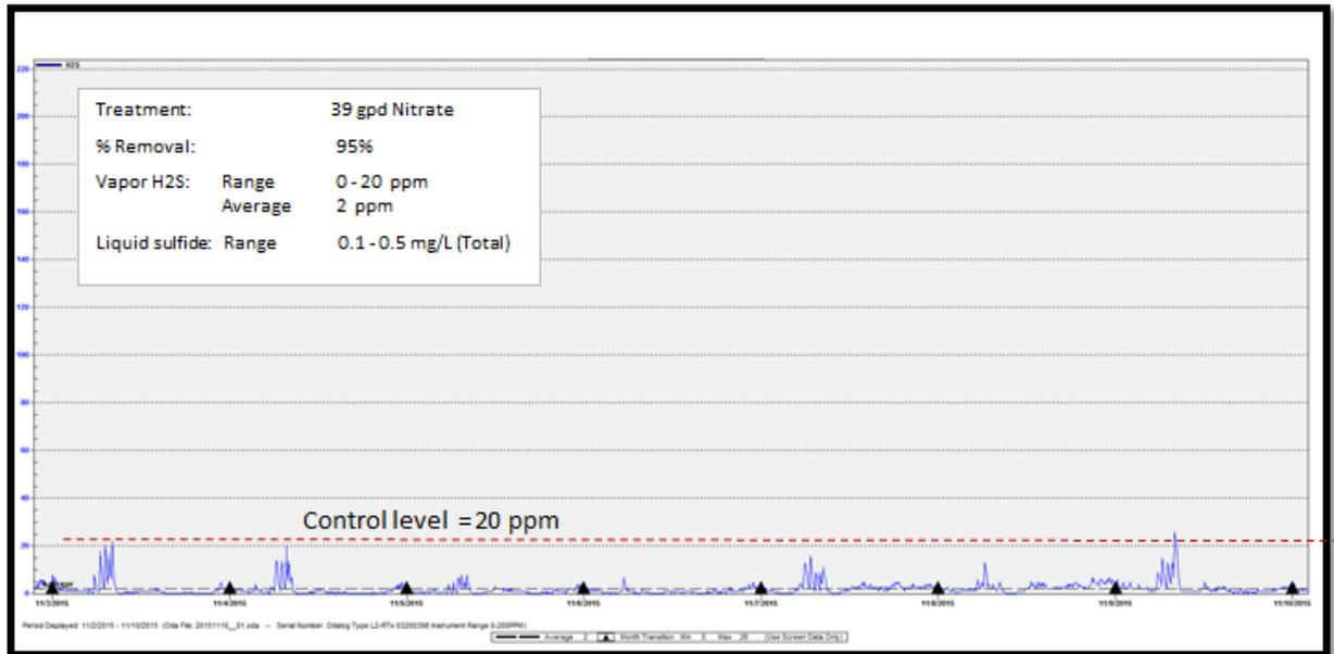
Results following the initial two Cloevis treatments are shown in Figures 12 and 13. The first treatment resulted in complete H<sub>2</sub>S suppression for 4-6 days, with the 20 ppm control level sustained for over 13 days (Figure 12). Results following a second (shorter) Cloevis treatment extended the length of complete suppression to 9-10 days, with control levels sustained for 18 days (Figure 13).
