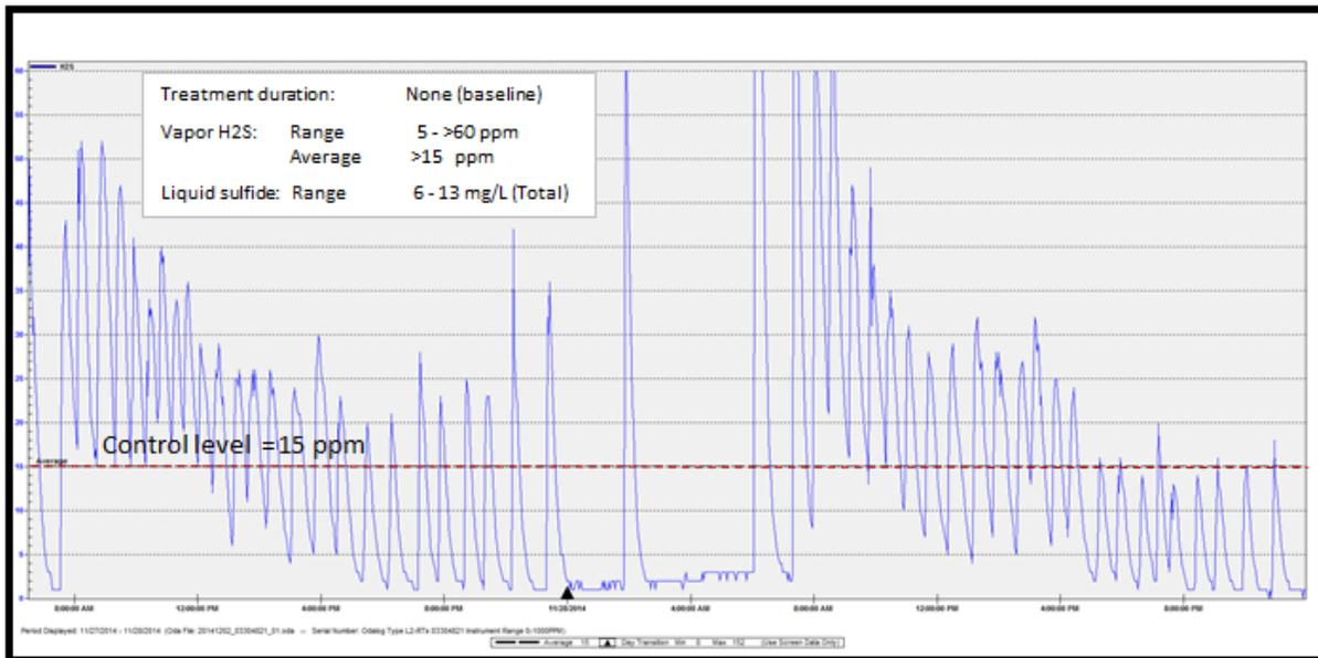
Figure 7 shows the H<sub>2</sub>S readings through the first 13 days following the initial 24-hr Cloevis treatment. The results show a 3-4 day period where H<sub>2</sub>S production is completely suppressed, followed by a slow recovery to where H<sub>2</sub>S control levels began to be exceeded on Day-8.
