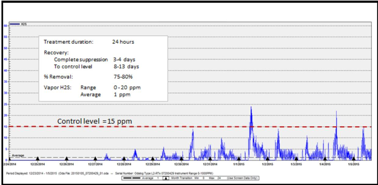
Figure 8 shows the H<sub>2</sub>S readings following a subsequent maintenance treatment. These results show continued control beyond the 13 day datalogging period (extending to 18-21 days).
