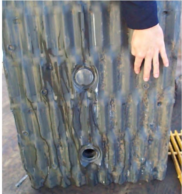
**Figure 39. Tower fill close-up after cleaning showing essentially complete deposit removal.**
