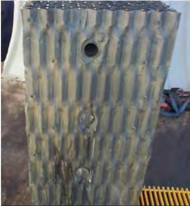
**Figure 38. Tower fill section after peroxide cleaning.**
