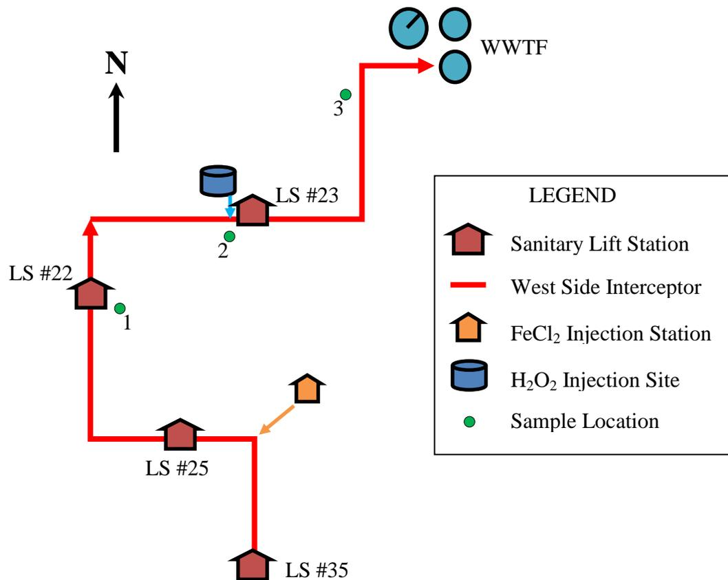
**Figure 1. PRI-SC Demonstration Flow Diagram.**
