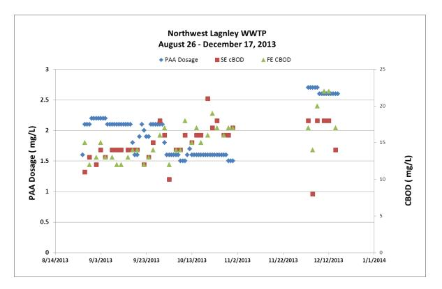
Figure 6: Comparison of cBOD of the final effluent and secondary effluent at various PAA doses.
