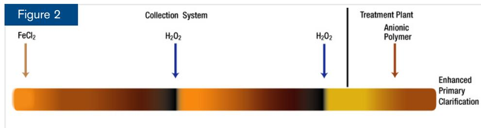
as it moves down the line. Intermittent hydrogen peroxide injection serves to regenerate the capturing agent thereby allowing additional sulfide to be absorbed downstream. Incorporating a final regeneration site at the treatment plant provides rapid oxidation of sulfides to very low levels, effectively reducing the H<sub>2</sub>S loading to the influent scrubbers. It also provides hydrous ferric iron that can be used for additional odor control in primary treatment or for enhanced clarification.
