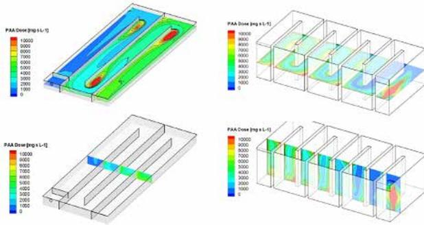
USP has unrivaled in-house CFD modeling expertise that can be used to optimize the injection, mixing and feed rates of PAA to meet the disinfection requirements of a facility.
