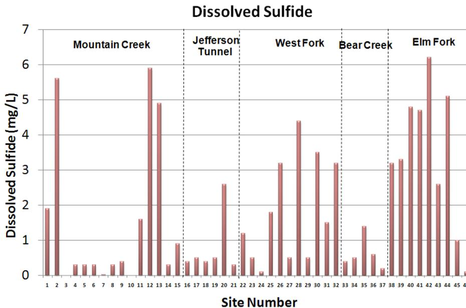
**Figure 3 - Dissolved Sulfide Grab Sample Data for TRA**
