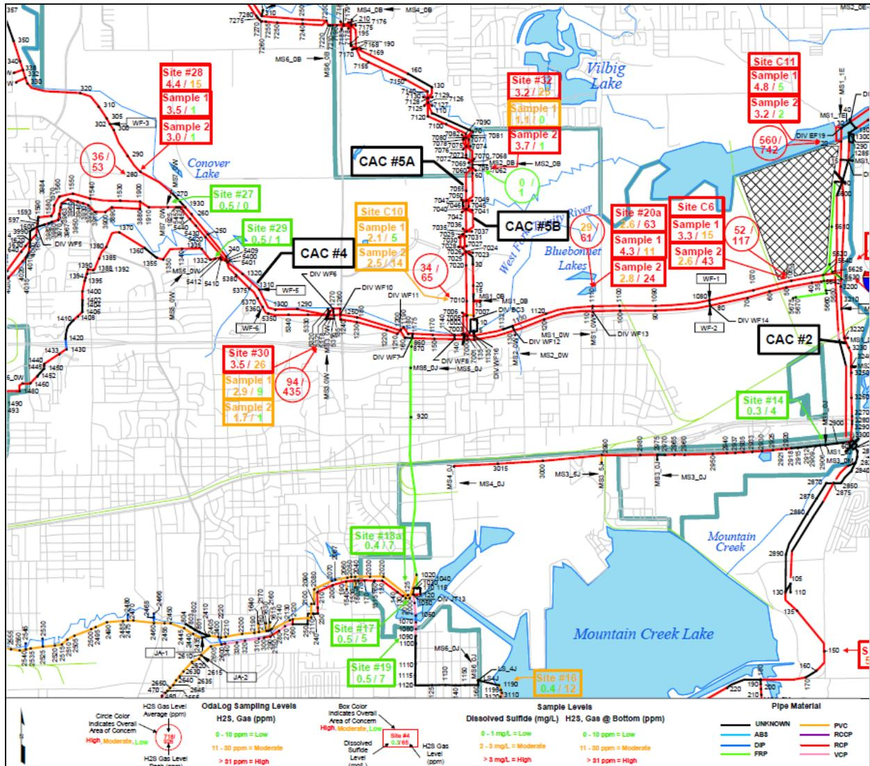
**Figure 6 - System Map with Dissolved Sulfide and H<sub>2</sub>S Data.**
