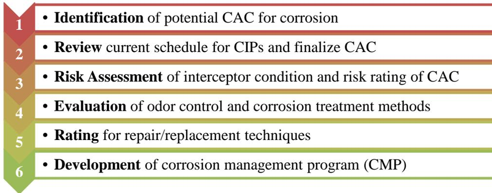
**Figure 1 - A Systematic Approach for Collection System Sulfide and Corrosion Management.**
