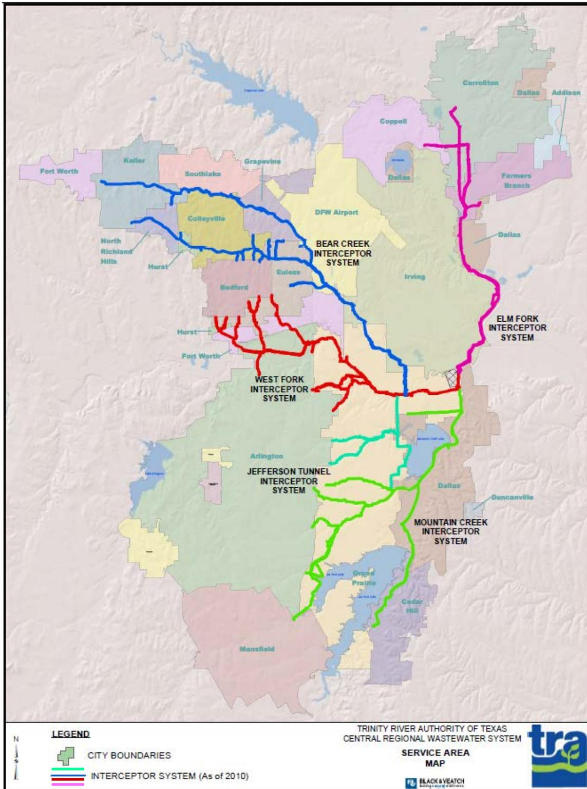
Figure 2 - Central River Wastewater System Interceptor Map of TRA.
